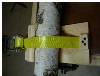
To support the other end of your log while cutting the tenon you can either make another clamp and secure it that way, or simply cut a support block similar to what is shown.
