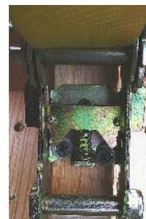
Mount one end of the long strap to the other end of the Base with screws, or you can secure the strap with a small piece of wood for added strength as shown.
