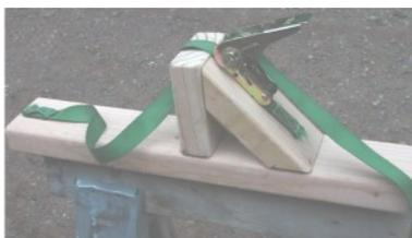
Use a ratchet strap that is easy to work. I like a sturdy ratchet with rubber grips. Some of the small ratchets are too flimsy, bend, are difficult to operate, and don't last long. The small strap that is already attached to the ratchet can be removed completely. Cut the hook end off of the long strap. Burn and melt both ends of the long strap so that they don't fray.
