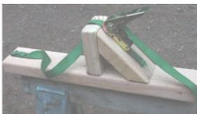
To attach the ratchet clamp onto the Brace, open it up completely and screw it onto the brace through the existing holes in the clamp. Use washers if necessary. Be sure that you put the ratchet far enough to the top so that it can be fully opened to release the strap. Shorten the strap if necessary and melt the end again to avoid fraying.
